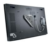
Barco's OverView KVD5521B is a high-performance, modular and cost optimized 55" LCD-panel, dedicated for use in tiled video wall applications. With an ultra-narrow bezel of 3.5 mm / 0.14", excellent colors and contrast, and a wide viewing angle, the OverView KVD5521B provides great value to entry-level and mid-range applications.
