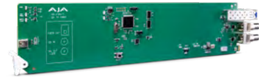
OG-FiDO-T $445 openGear 1-Channel 3G-SDI to Single Mode LC Fiber Transmitter, with SDI Loop Out
